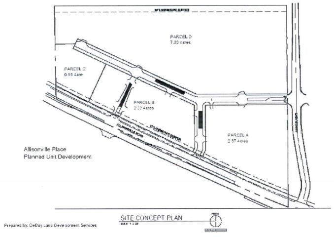
This site concept plan for the Allisonville Place Planned Unit Development shows the approximate location of the right-n/right-out curb cut on Allisonville Road. The exact location of the curb cut will be established with the approval of the Final Development Plan for Parcel A. The location of the line dividing Parcels B and C will be established with the Final Development Plans for those parcels.
