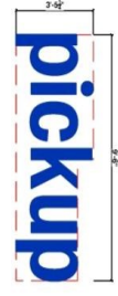
C1 PICKUP SIGN NBS LOW PROFILE REVERSE HALO LT 3" DEEP POLYCARBONATE LETTERS MOUNTED TO 1/2" X 1/2" X 1/2" ALUMINUM FACE COLOR: BLUE (PMS 286C) TOTAL 263.3 S.F.
