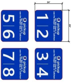
A4 PICKUP SIGN PARKING SPACE NUMBERS NBS SIGN POLE AND BASE TO BE CONSTRUCTED PER DETAIL B1 ON C-701 TOTAL 43.8 S.F.
