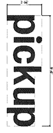
C1 PICKUP SIGN 4'-6" HIGHS LOW PROFILE REVERSE HALO LIT 3" DEEP POLY-CARBONATE COLOR: BLUE (PMS 288C) TOTAL: 50.3 S.F.
