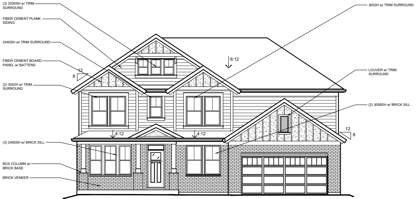
FRONT ENTRY w/ BRICK VENEER AVAILABLE w/ LOW OR HIGH BRICK SIDES AND REAR
