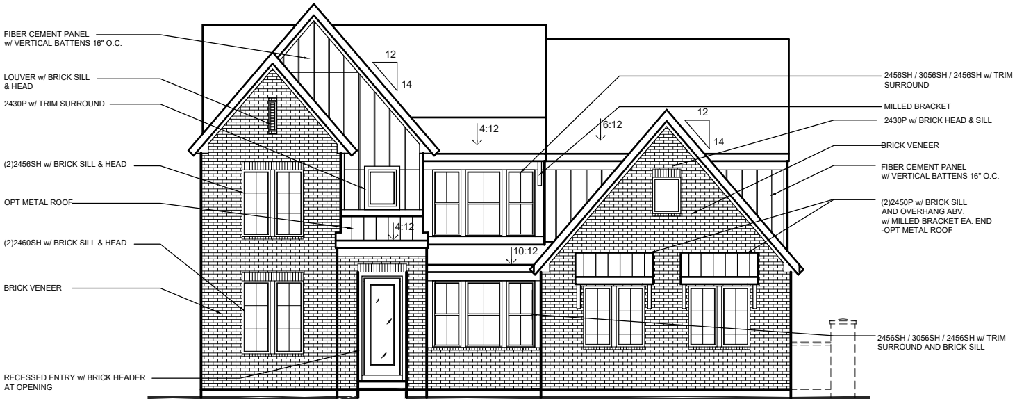
SIDE ENTRY w/ BRICK VENEER w/ OPT. WING WALL w/ BRICK BASE (AVAILABLE w/ LOW or HIGH BRICK SIDES & REAR)
