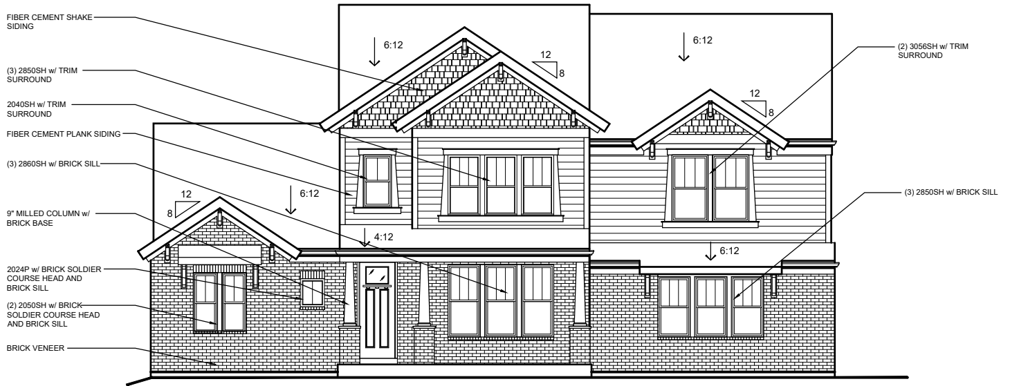
SIDE ENTRY w/ CULTURED STONE VENEER AVAILABLE w/ LOW OR HIGH BRICK SIDES AND REAR
