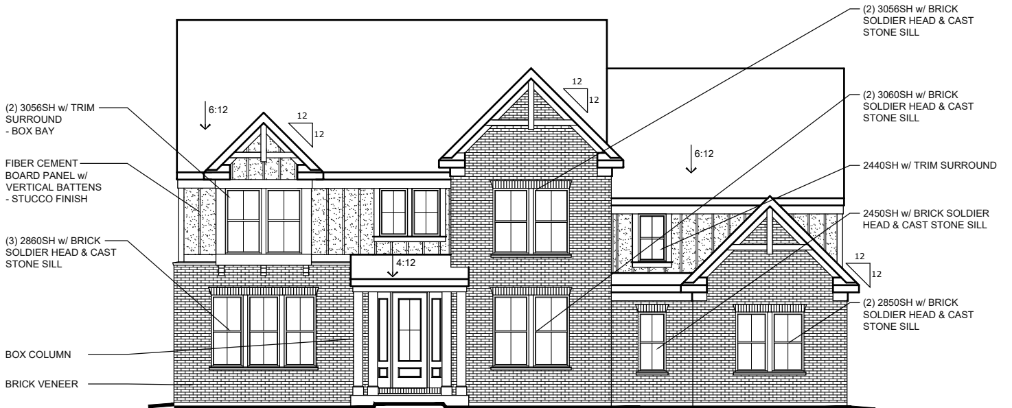
SIDE ENTRY w/ BRICK VENEER w/ INCLUDED FRONT PORCH AVAILABLE w/ LOW OR HIGH BRICK SIDES AND REAR
