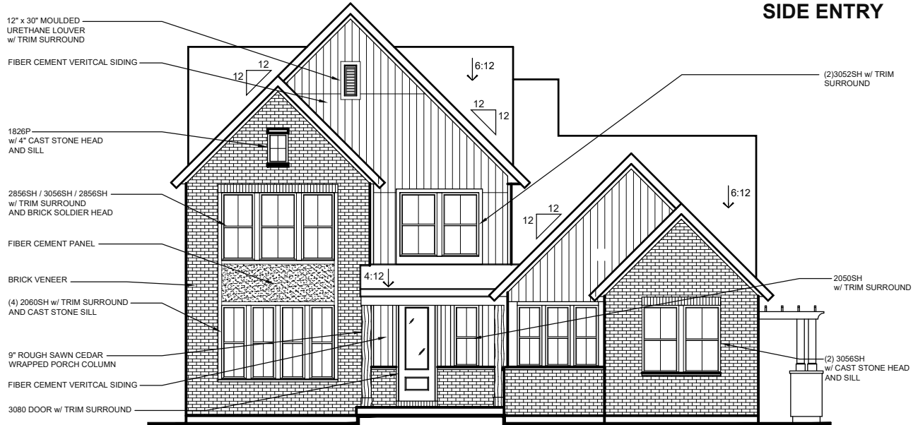
w/ BRICK VENEER w/ OPT. RSC TRELLIS & BRICK BASE WING WALL (AVAILABLE w/ LOW OR HIGH BRICK SIDES)
