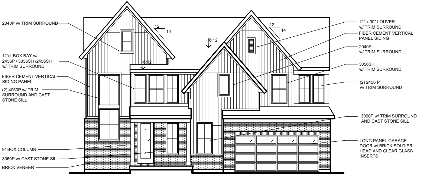
FRONT ENTRY w/ BRICK VENEER (AVAILABLE w/ LOW or HIGH BRICK SIDES & REAR)
