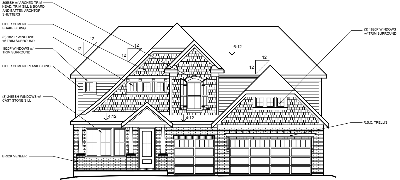
THREE-CAR INTEGRATED FRONT ENTRY GARAGE w/ BRICK VENEER AVAILABLE w/ LOW OR HIGH BRICK SIDES
