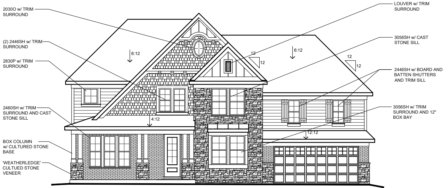
FRONT ENTRY w/ BRICK AND CULTURED STONE VENEER AVAILABLE w/ LOW OR HIGH BRICK SIDES AND REAR
